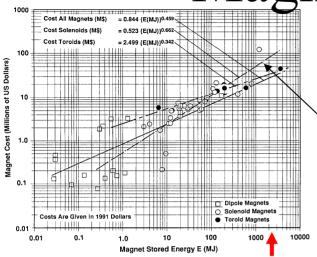
Figure 1. Superconducting Magnet Costs Versus Magnet Stored Energy.
