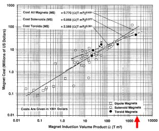
Figure 2. Superconducting Magnet Cost Versus Field-Magnetic Volume Product.
