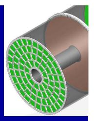
3 10<sup>9</sup> volume pixels. 224 points per track. Single-point resolution 50 - 100  $\mu$ m r- $\phi$ , 400  $\mu$ m r-z [cos $\theta$ ] < 0.985 (TPC) [cos $\theta$ ] < 0.996 (FTD)
