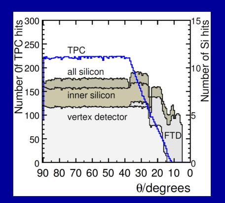
Complete TPC coverage to  $37^{\circ}$ VTX + SIT + FTD + SET + ETD => precision, redundancy and coverage to  $|\cos\theta| = 0.996$ .
