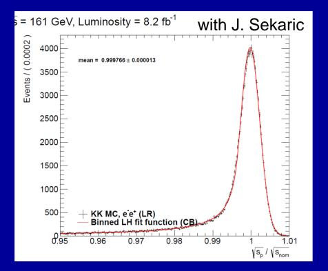
ILC detector momentum resolution (0.15%), gives beam energy to better than 5 ppm statistical. Momentum scale to 10 ppm => 0.8 MeV beam energy error projected on  $m_W$ . (J/psi)
